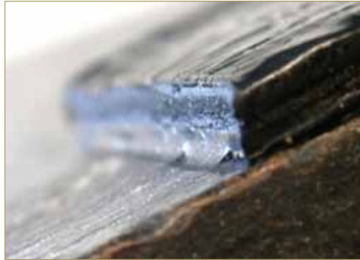
WATER PROOF SHEETS - Determination of high temperature flowing Standard UNI 8202, Part 16
