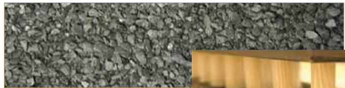
ADESO POLYGLASS MEMBRANE After 50 brushing cycles
