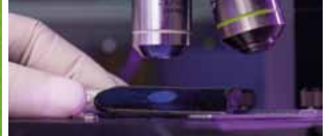
THICKNESS - Fluorescence microscope at 250X magnification. Standard UNI EN 1849-1
